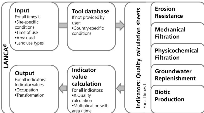
**Figure 3-2 LANCA® structure**
